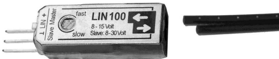
Figure 3: LIN 100 connection with the optical fibre
