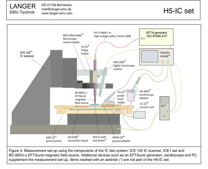
The field source is attached to the rotary unit of the ICS 105 IC scanner using the SH 01 probe holder (**Figure 5**). The probe holder has the function of collision control: If the field source encounters resistance while moving downwards (field source meets the IC), the field source in the probe holder will move upwards. This displacement can be detected by the ICS 105 IC scanner and the movement is stopped.
