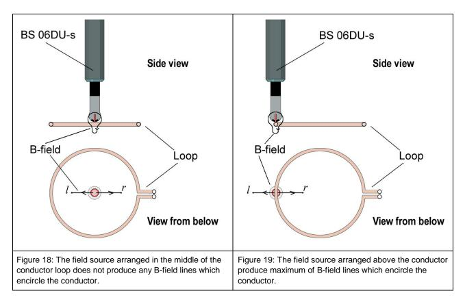
The field-line bundle is inhomogeneous at the outlet area of the field source. The field lines first run vertically downwards over a small area and below the exit point horizontally to the surface of the DUT. The flux density decreases with an increasing distance h from the coil.
