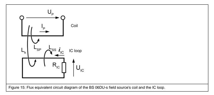
The current  $i_P$  in the coil generates a vortex magnetic field. The share of the vortex magnetic field which penetrates the IC loop is assigned to the principal inductance  $L_h$ . The principal inductance  $L_h$  mediates between the current  $i_P$  of the field source and the flux  $\Phi$  which flows through the IC loop.
