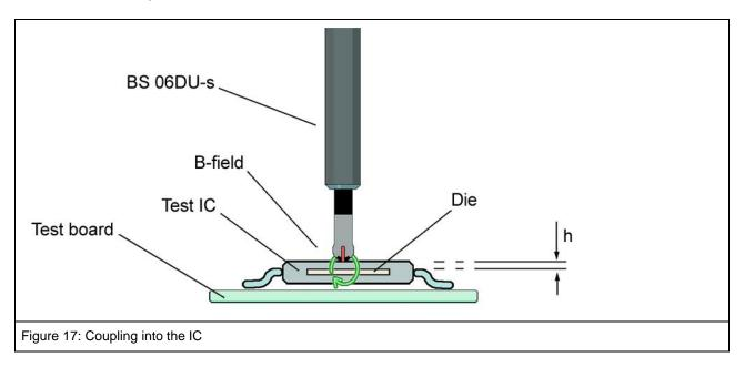
The field-line bundle of the field source penetrates the die in an orthogonal direction (**Figure 17**). In particular loops that are orthogonal to the plane of the die (vertical) are penetrated by the field line bundle. Either voltage or current is transferred in the loops depending on the type of coupling (**Figure 17**).
