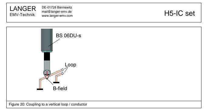
Similarly, the field source has to be placed nearly to the vertical loop (**Figure 20**) to allow the field lines encircle the loop's conductor.
