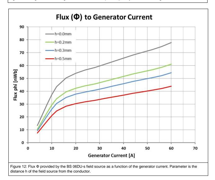
The effective flux  $\Phi$  can be obtained from the diagram in **Figure 12** for each specific individual case. The required current I<sub>P</sub> can be calculated from the voltage U<sub>P</sub> that is set at the EFT/burst generator according to Eqn 1. The distance h corresponds to the distance between the IC loop and the field source.
