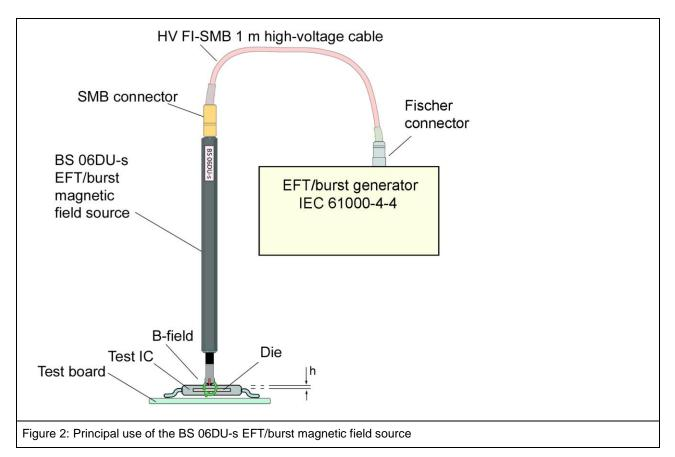
The coordinates of the field source can only be detected with low precision if the field source is guided by hand over the device under test (DUT, such as an IC, component or printed circuit board). A defined point on the IC's surface can only be approached roughly and is almost impossible to reproduce. The field source cannot be guided safely enough by hand if the die is exposed. The IC may be damaged.
