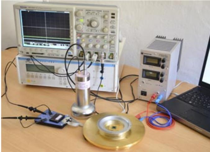
Figure 18 – Measurement set-up with the device under test in the test adapter
