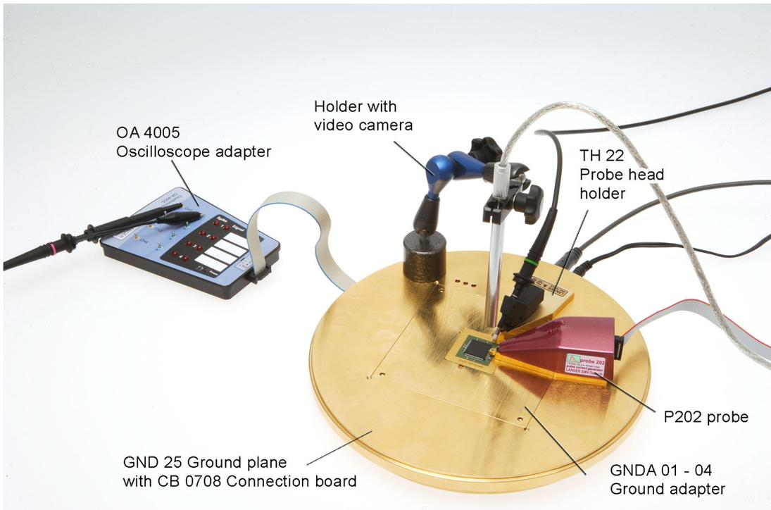
Scheme measurement set-up Set ICE1 with extern devices
