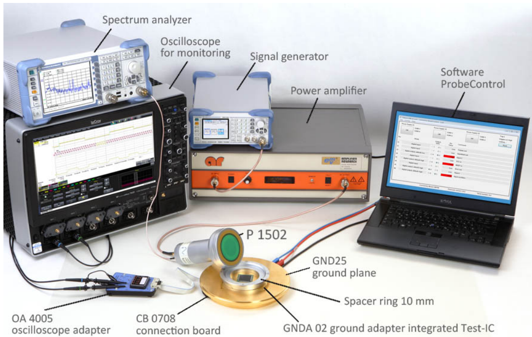
Measurement set-up with P1502 RF E-Field source
